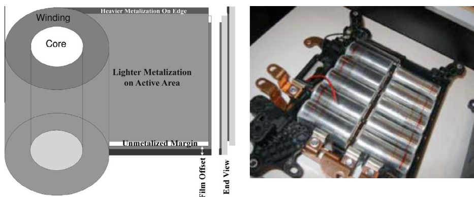
Fig. 2. (Left) Single-section winding showing more heavily metallized edges region, lightly metallized active region, and an unmetallized margin. The two layers are offset so that the heavily metallized region at the top protrudes beyond the layer below. (Right) A bank of metallized capacitor windings found in a typical hybrid electric vehicle.
